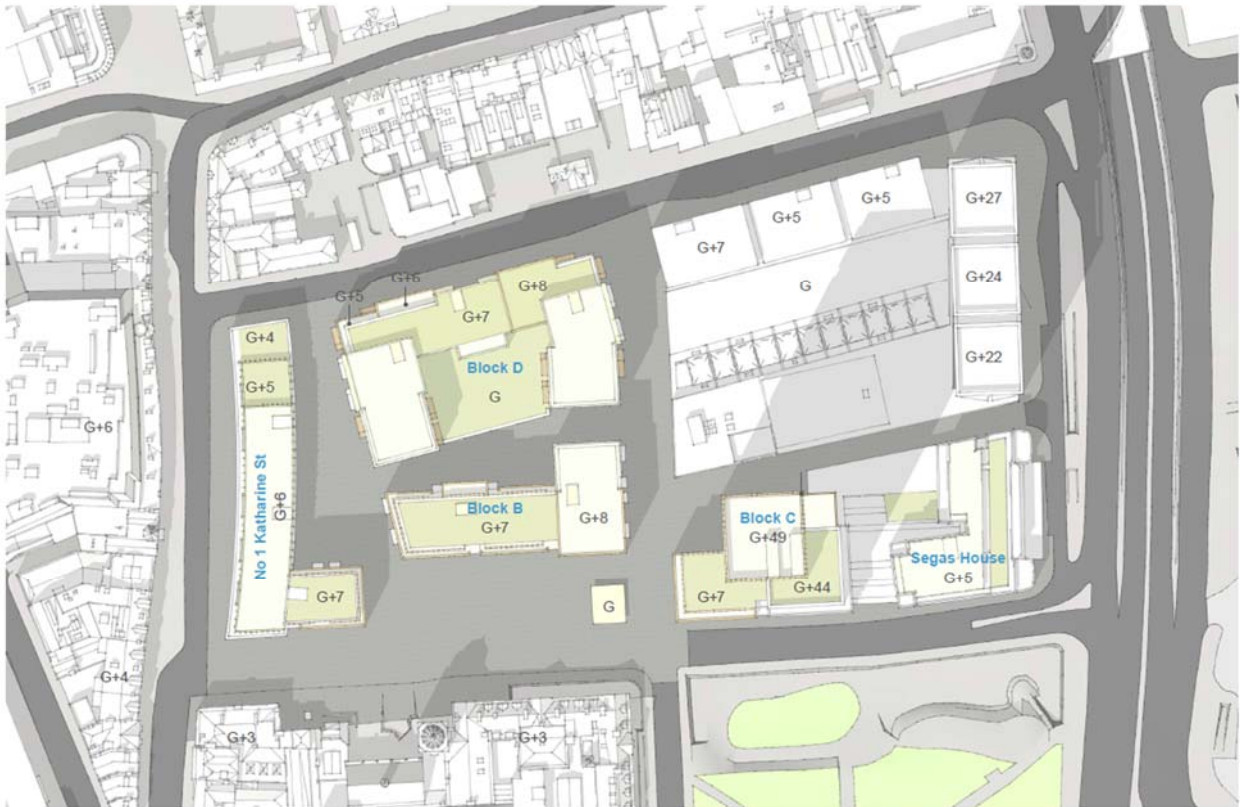
Heights to Block D still under review, for current purposes the two wing elements are shown as Ground + 8 storeys (facing Thomas Turner Place) and Ground + 10 storeys (facing St George's Walk) respectively.
